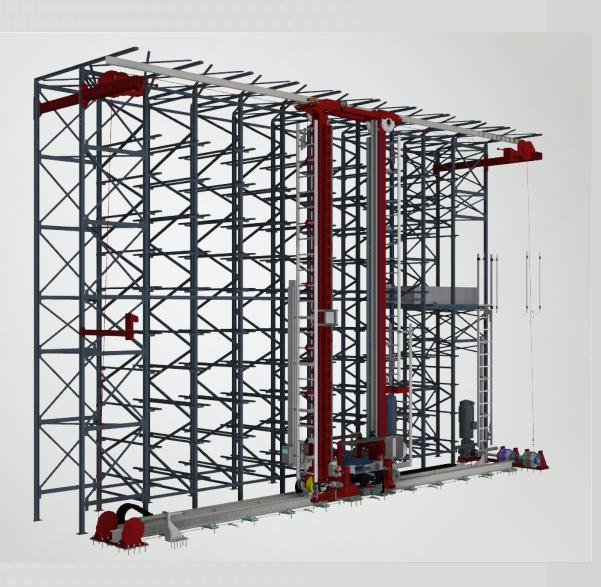
The Green Tire automatic warehouses with Cartesian and Cartesian VX are the ideal solution for brownfield applications, where plants with narrow or poorly distributed spaces require the maximum capacity to be obtained in terms of Green Tire quantity stored and flows.
