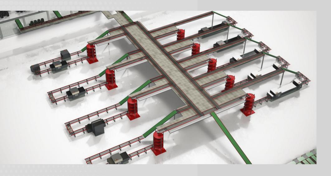
From the curing press, the tire is ready for the quality control phase. The conveyor system takes the tires to the manual inspection stations (visual control) and to the automatic quality control phase with special machinery (testing machines). Each manufacturer follows a specific set of inspection protocols and quality tests on products, in order to
