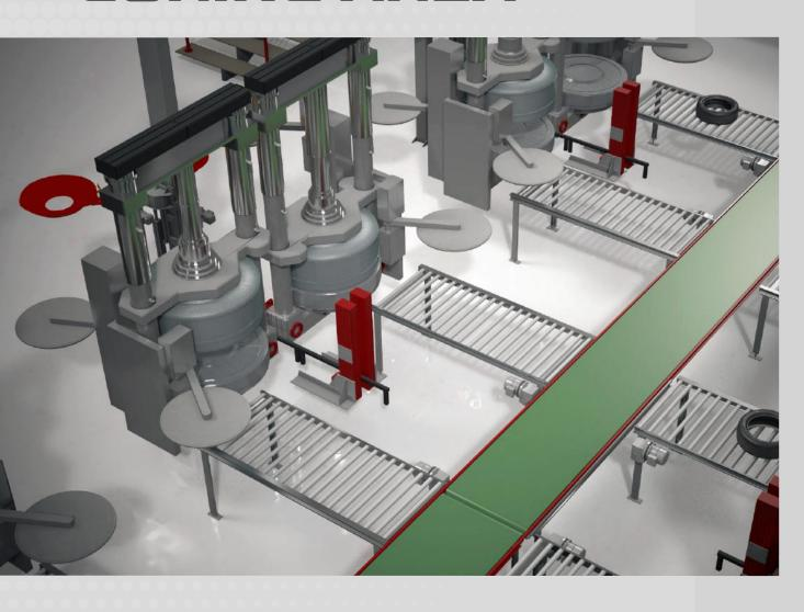
The vulcanisation process is used to obtain the final shape of the tire and the design of the tire thread. Vulcanisation is carried out in the press areas, using heat and pressure in tire moulding. When the Green Tire is called to feed the presses, the tires are treated in the painting machine, designed for painting green tires, both inside and out, with special emulsions that enable easy detachment Green Tire following vulcanisation in the press.
