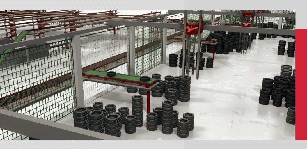
From the inspection area, the tires are conveyed for storage and palletizing. Palletizing starts with the Gantry, designed and built to manage the tires for intensive storage.
