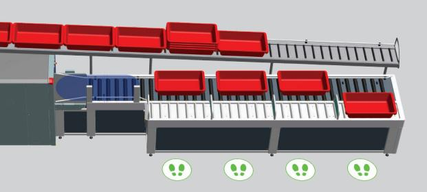
Trays are moved through a high-speed exchange system. The time needed to make such a deviation is less than 1.5 seconds. This special system guarantees rapid response times without impacting the tray path (tray jamming is prevented).
