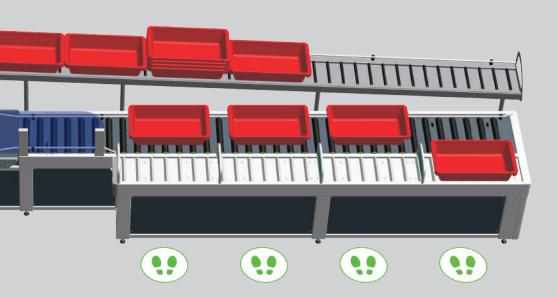
The «Queue Beater» allows queues to be distributed in an ordered and efficient way, increasing throughput and easing inspections by operators. Once baggage has been checked, empty trays return to the start by a raised gravity
